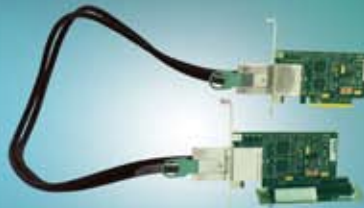
PCIe x8 host and target adapters in 2-slot backplane (OSS-KIT-EXP-8000-2M)
