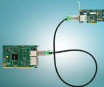
PCIe x4 host adapter and expansion board (OSS-KIT-EXP-1500-2M)
