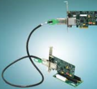
PCIe x4 host and target adapters in 2-slot backplane (OSS-KIT-EXP-3500-2M)
