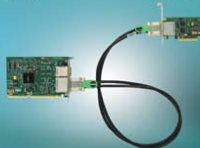
PCIe x8 host adapter and expansion board (OSS-KIT-EXP-7500-2M)
