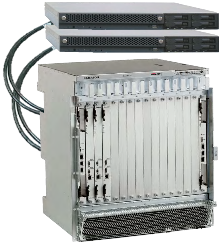
A hybrid system utilizing dual motherboard-based servers and an ATCA-based I/O sub-system
