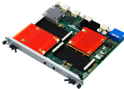
Emerson Network Power ATCA CPU blade
