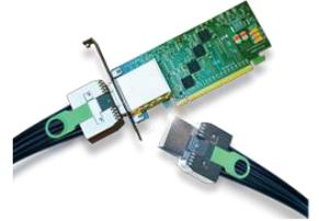
latency of cable connections. Gen3 x16 operates at speeds up to 128Gb/s. The CUBE2 can also connect to a Thunderbolt-enabled computer through a Thunderbolt cable. Compared to Thunderbolt 1, Thunderbolt 2 doubles the speed of the data path to 20Gb/s and increases the bandwidth of the Display Port to 20 Gb/s. The Thunderbolt 2 Option Card installs in the CUBE chassis and converts the Thunderbolt bus from the computer to PCIe.
